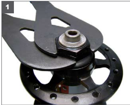
1. Using two 19mm cone wrenches, turn counter clockwise to loosen and remove the lock and adjusting nut.
