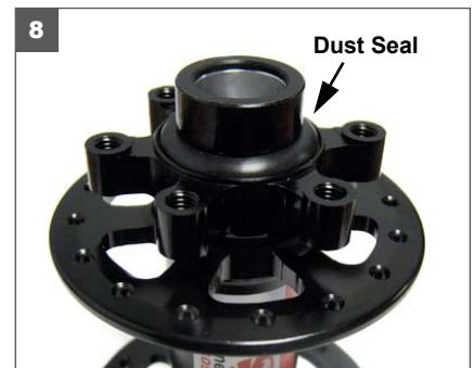
8. Finally slide the remaining dust seal over the end cap on the disc side.
