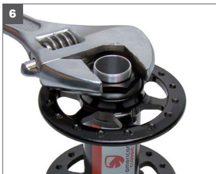
6. Thread the 22mm adjusting nut with dust seal attached onto the end of the 15mm thru-axle and tighten with a wrench. Tighten the adjusting nut until there is no play and back off one quarter rotation.
