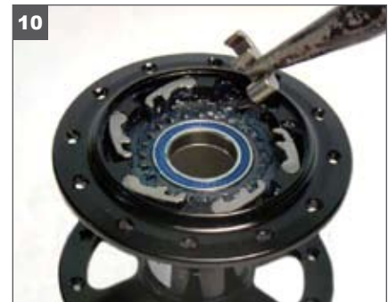
10. With a thin layer of clean grease coating the top of the cam plate, install all 6 pawls. Once completed the pawls should freely engage in unison with the cam plate.
