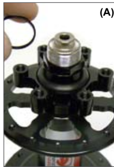
A. Some hubs have a 1.5mm axle spacer.
