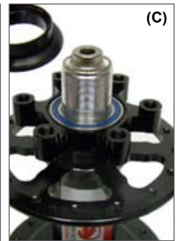
C. Remove spacer with attached dust seal.
