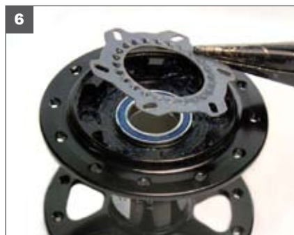
6. Remove cam plate.
